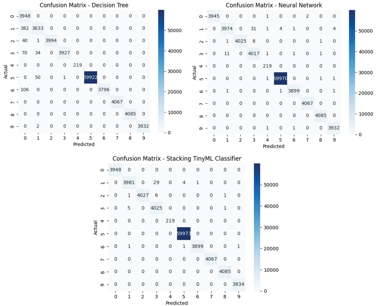
Fig 2. Confusion matrices for the DT, NN and stacking TinyML models.
