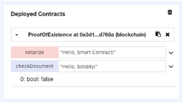
Figure 7-15. Entering a different string other than the original string will yield a result of false
